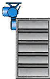
MXb and worm gearbox mounted to damper
