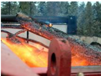
Figure 5— Photo shows results when the airflow is broken; a log smolders above the air curtain.
