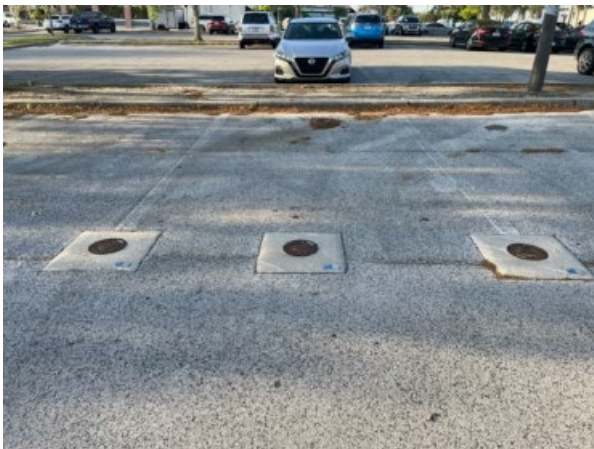
Photo 9: Three monitoring wells observed on the north central portion of the site
