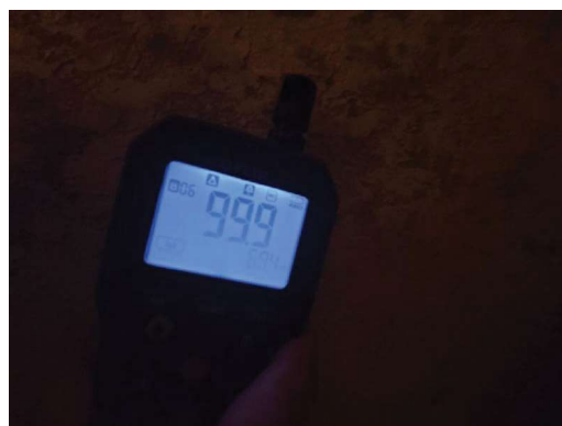
Interior Northwest Bedroom Closet Drywall wall Elevated moisture content (99.9%)
