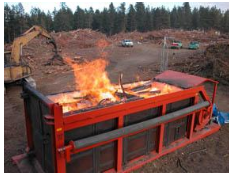
Figure 1—ACD in full operation (no visible smoke).
