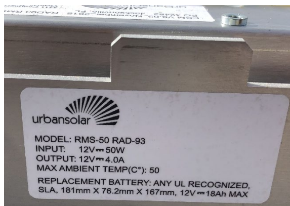
FIGURE 9: URBAN SOLAR RMS-50 NAME PLATE WITH MAXIMUM TEMPERATURE RATING OF 50°C (122°F)
