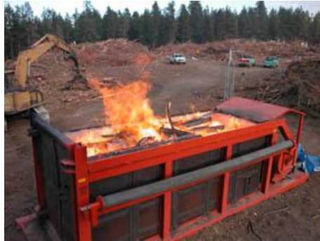
Figure 1—ACD in full operation (no visible smoke).
