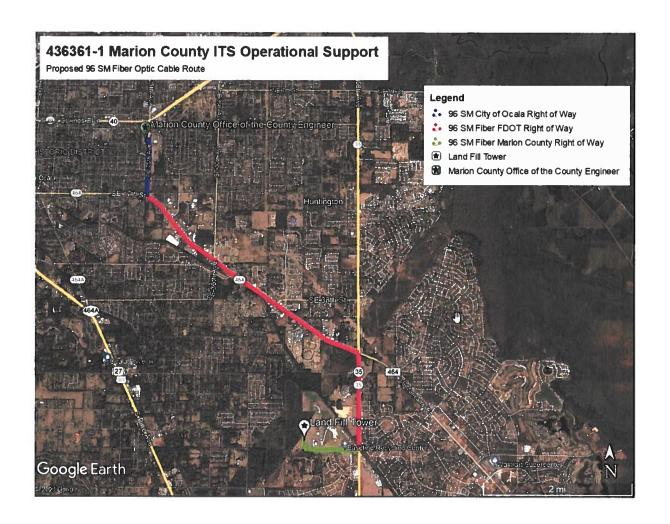
Project includes installation of fiber optic cable from the Marion County Office of the County Engineer to the Land Fill Tower in the Marion County Solid Waste Facility. The cable will run south down SE 25<sup>th</sup> from the Marion County Office of the County Engineer, east along SR 464, south down SR 35, then west along Laurel Rd to the Land Fill Tower in the Marion County Solid Waste Facility.
