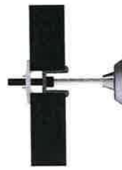
N5 Bonding Clamp: Insert clamp between module torques to 20 ft-lb.
