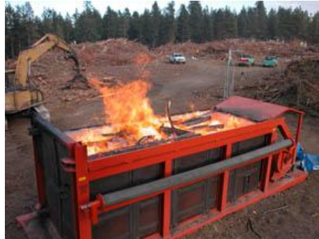
Figure 1—ACD in full operation (no visible smoke).
