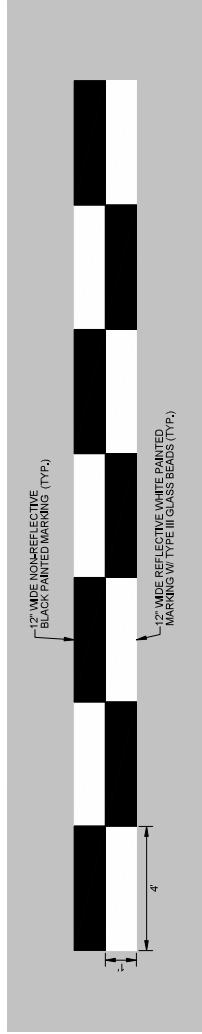
1 SERVICE ROAD STRIPING DETAIL
