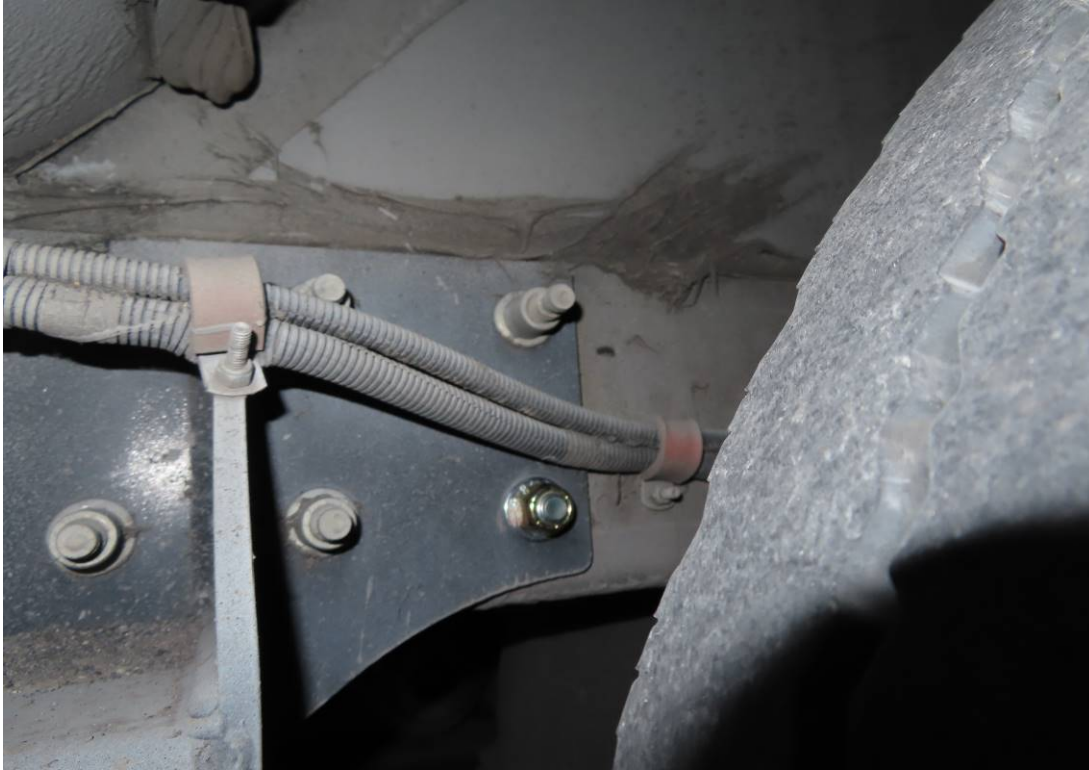
BROKEN HUCK BOLT REPLACED (11,491 TEST MILES)
