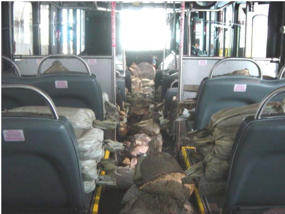
BUS LOADED TO 2.5 TIMES GVL (28,125 LBS)
