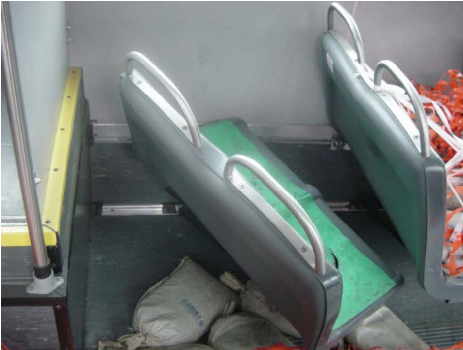
BROKEN SEAT FRAME (5,500 TEST MILES)
