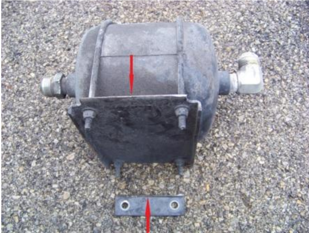
FAILED AIR TANK MOUNTING BRACKET (8,074 TEST MILES)
