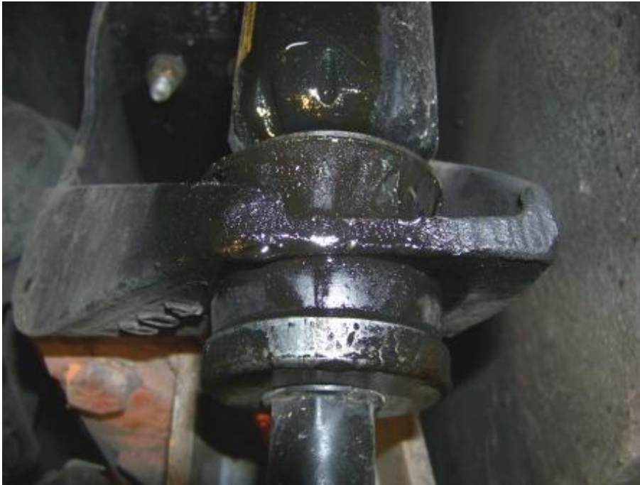
FRONT SHOCK LEAKING OIL (4,379 TEST MILES)
