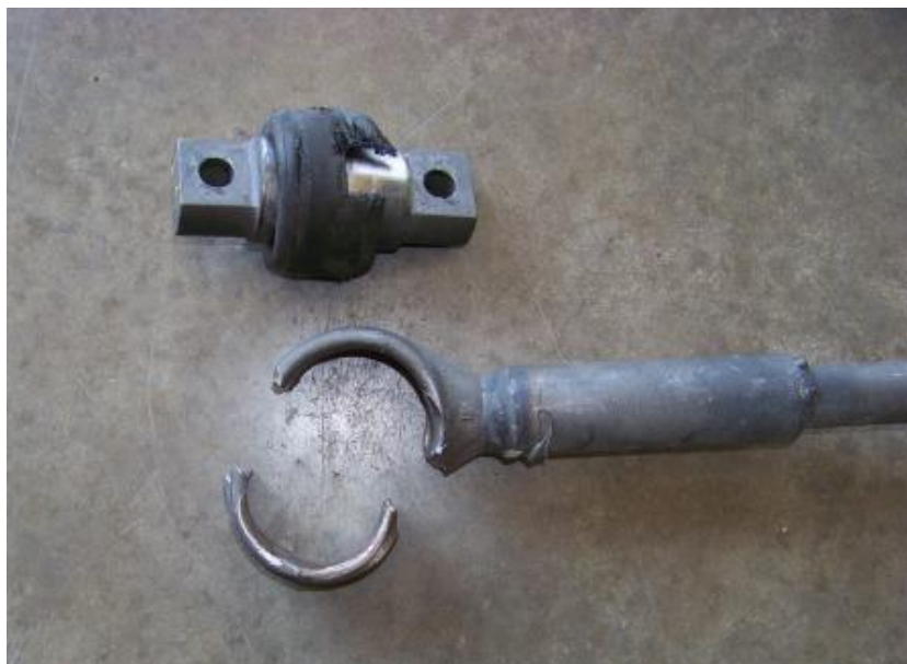
BROKEN TRACK ROD EYE (3,785 TEST MILES)
