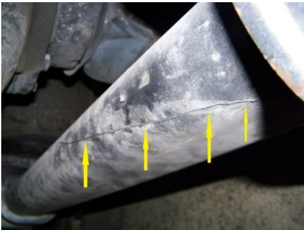
CRACKED TRANSVERSE BAR IN REAR, LOWER CONTROL ARM ASSEMBLY (3,785 TEST MILES)
