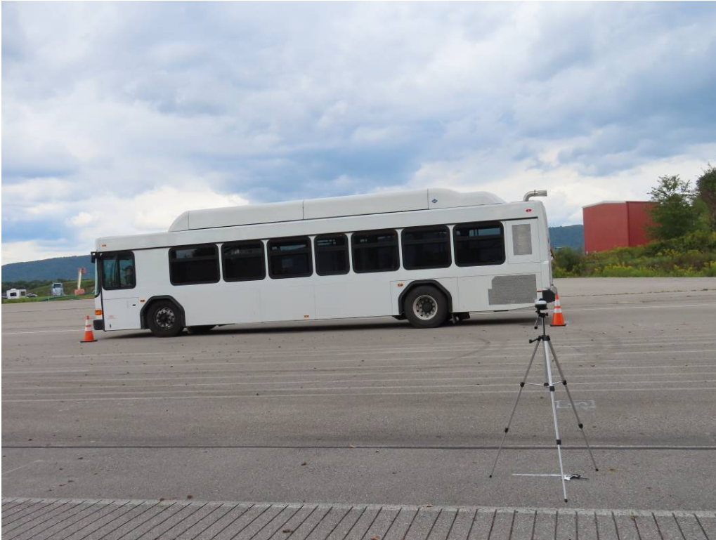
TEST BUS UNDERGOING EXTERIOR NOISE TESTING
