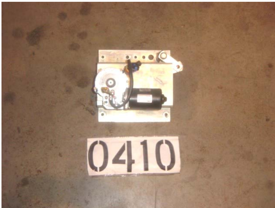
WIPER MOTOR REMOVAL AND REPLACEMENT (0.50 MAN HOURS)
