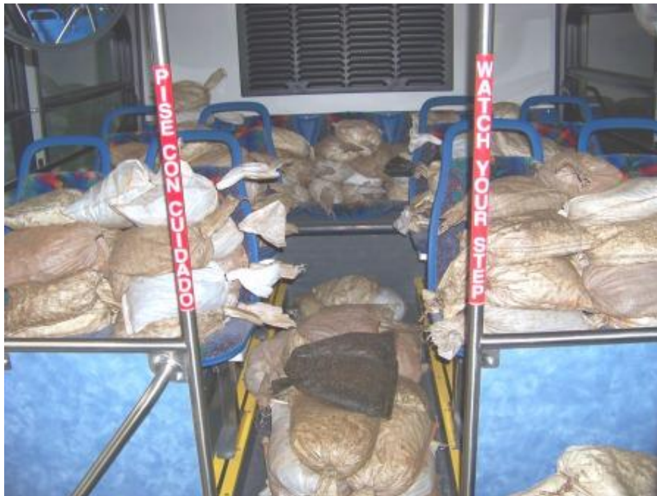
BUS LOADED TO 2.5 TIMES GVL (16,575 LBS)
