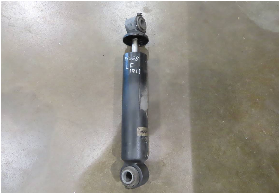
FRONT SHOCK LEAKING (11,491 TEST MILES)
