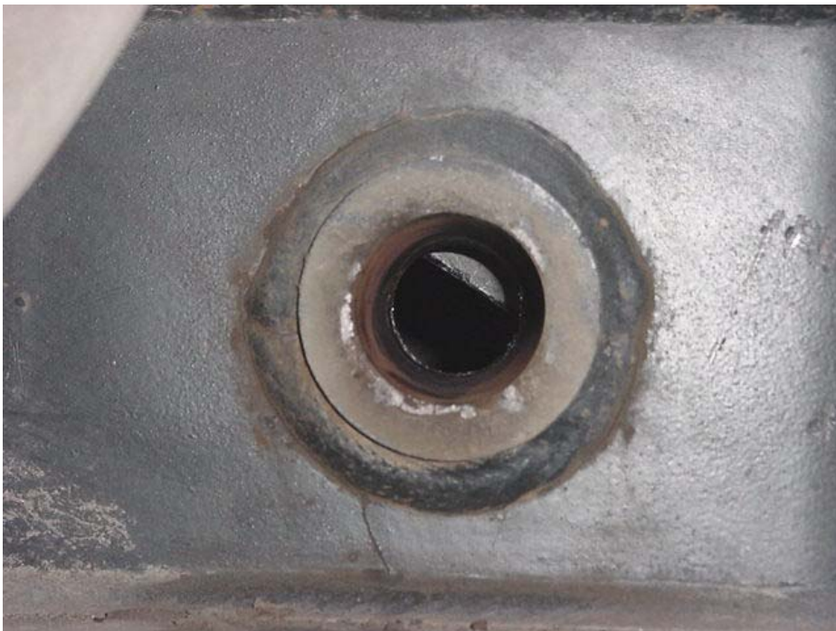
CRACKED H-BEAM ANCHOR POINT (12,743 TEST MILES)
