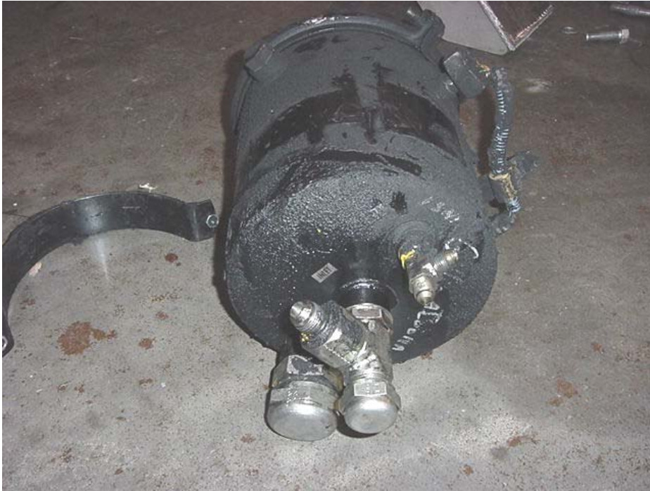
CRACKED HYDRAULIC RESERVOIR (12,487 TEST MILES)
