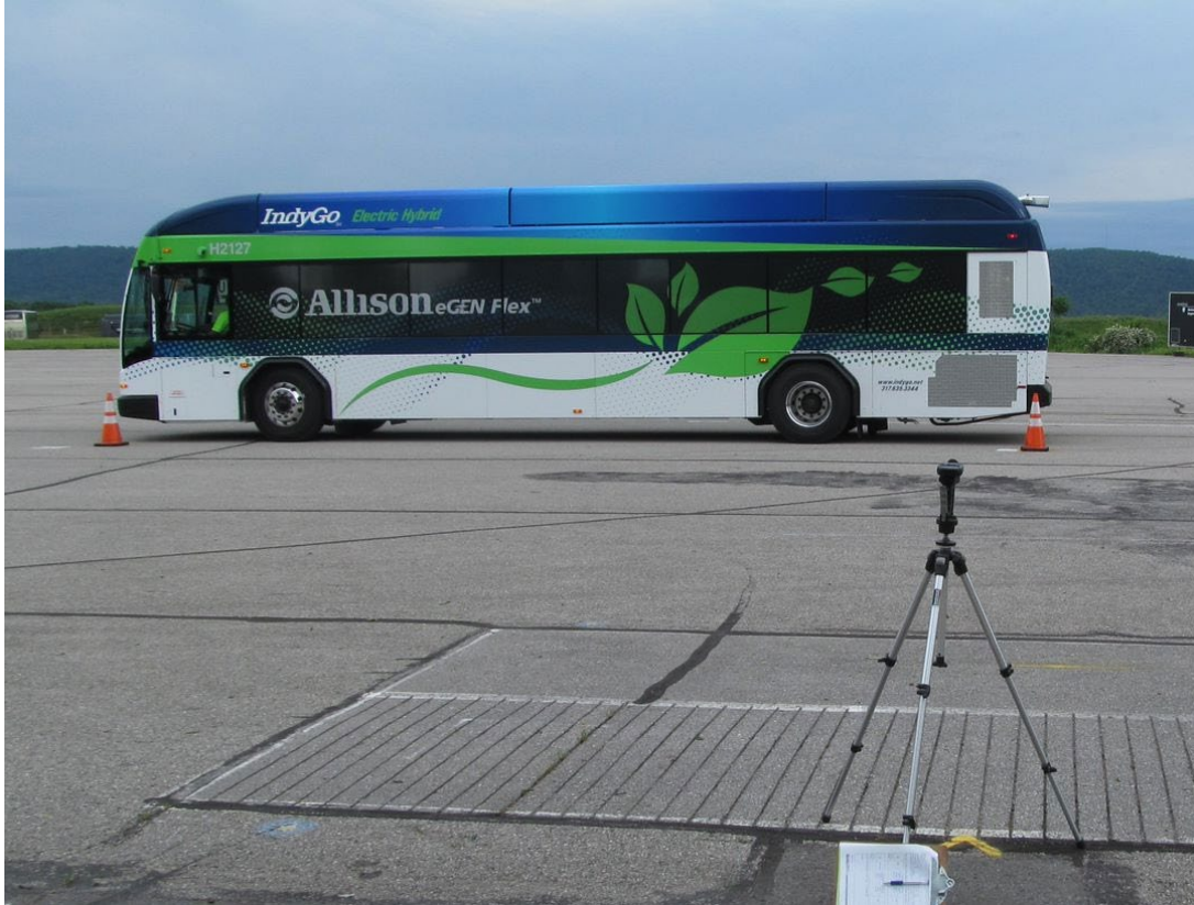
TEST BUS UNDERGOING EXTERIOR NOISE TESTING
