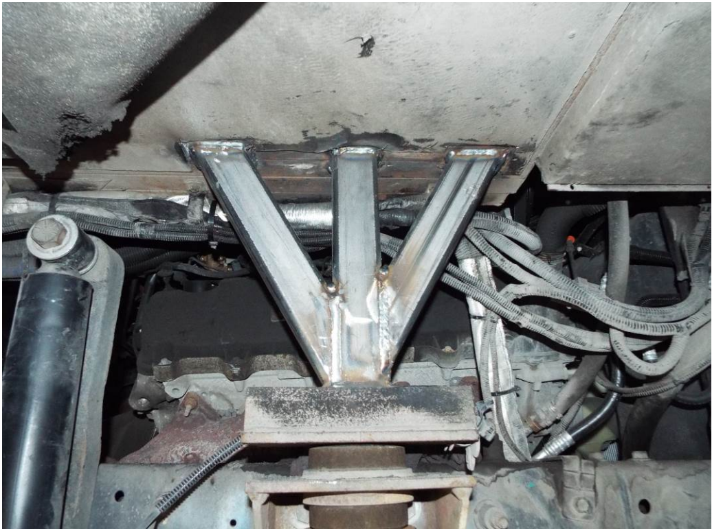
FRONT BODY MOUNTS REPAIRED (2,980 MILES)
