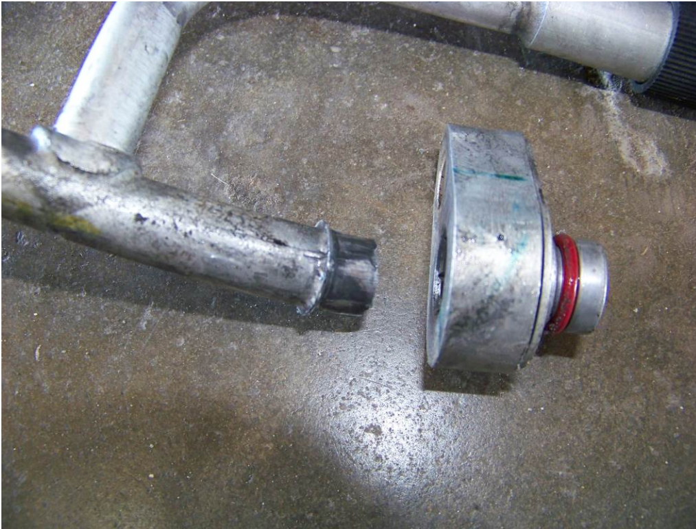
BROKEN A/C LINE (5,230 MILES)
