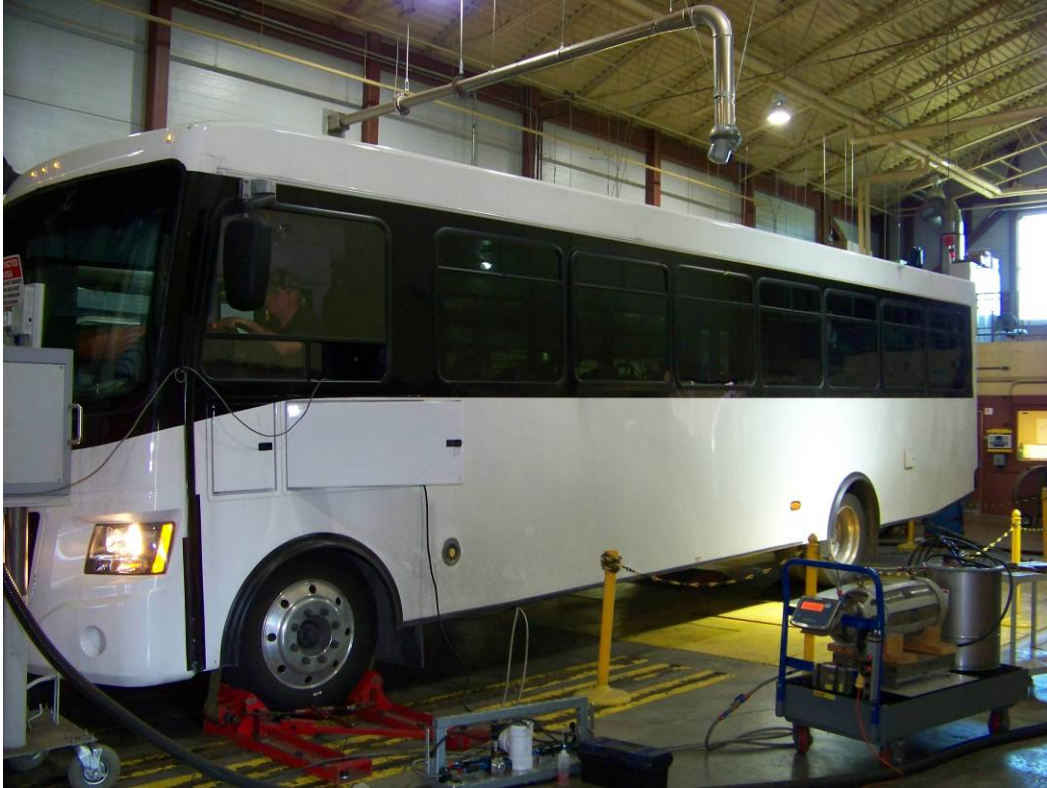
BUS TESTED ON CHASSIS DYNAMOMETER FOR PERFORMANCE, EMISSIONS AND FUEL ECONOMY
