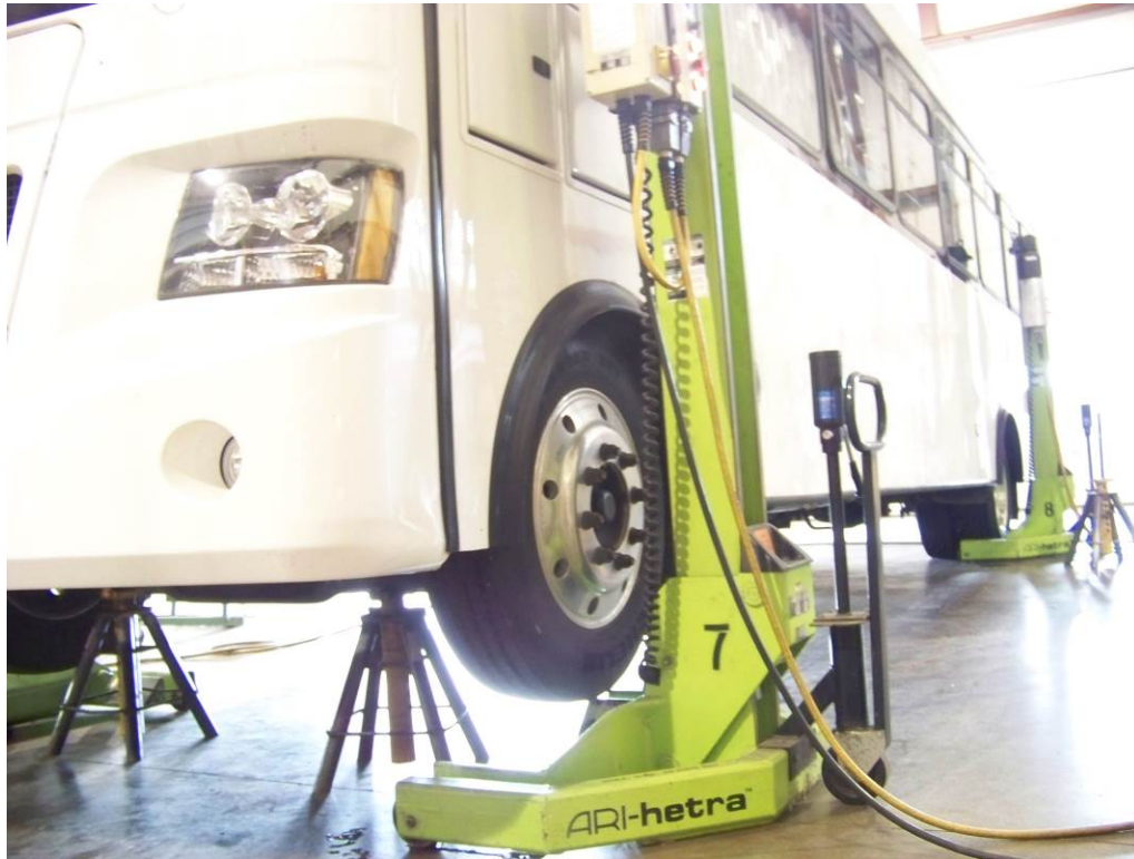
FRONT OF BUS ON JACK STANDS
