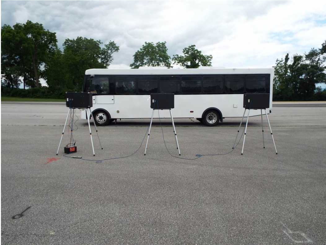
TEST BUS SET-UP FOR 80 dB(A) INTERIOR NOISE TEST
