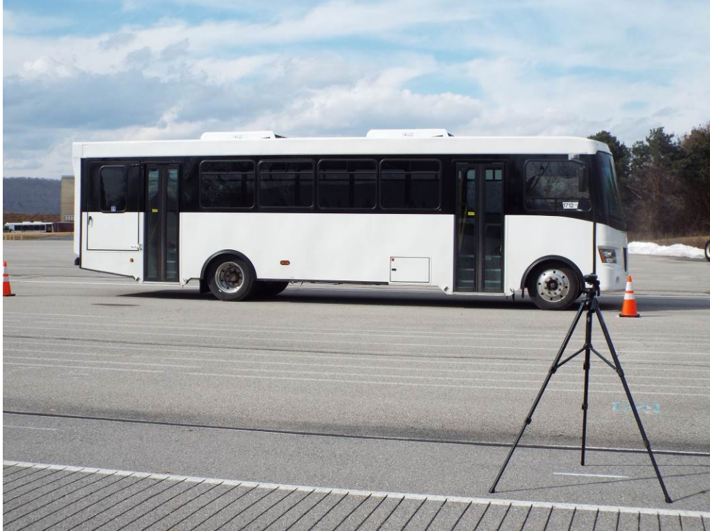
TEST BUS UNDERGOING EXTERIOR NOISE TESTING
