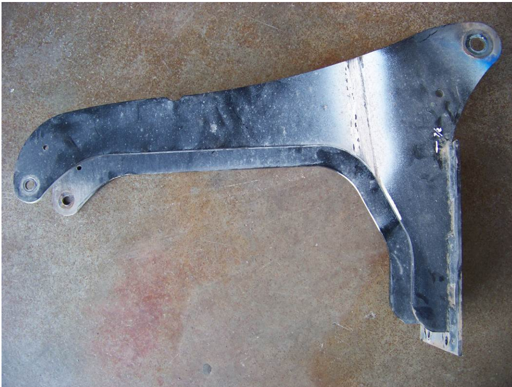
CRACK ON OUTSIDE FACE OF LEFT, REAR MORRYDE SHACKLE (6,406 MILES)
