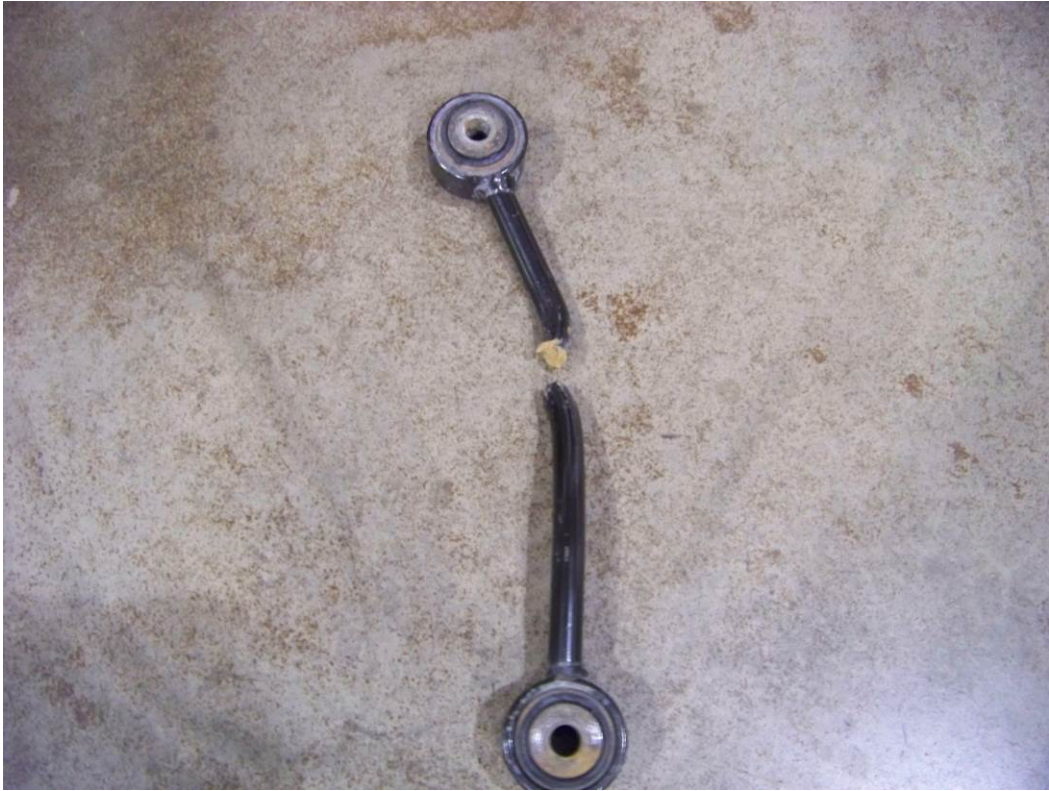
BROKEN FRONT SWAY BAR (322 MILES)
